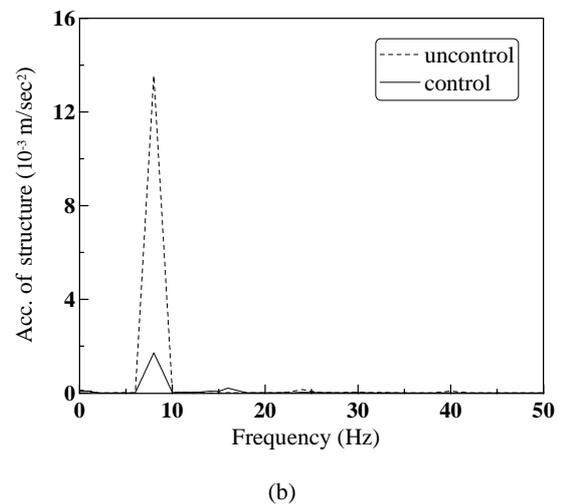
Fig. 7 Response of the anti-vibration under an excitation at 8Hz, (a) time domain; (b) frequency domain.
