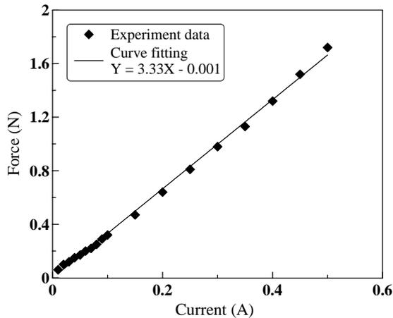
Fig. 4 The relation between the thrust of VCM and the applied current
