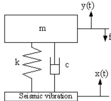
Fig. 2 Schematic of the active vibration isolation system.
