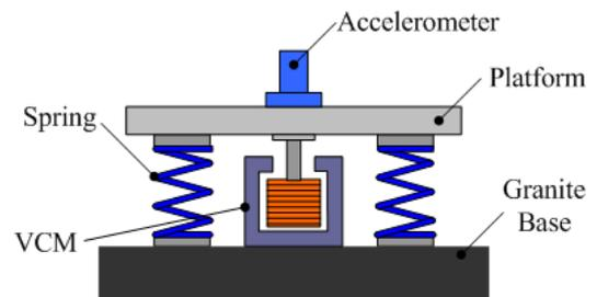
Fig. 3 The setup of the active vibration isolation system
